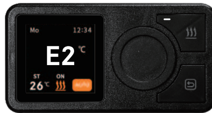
Temperature sensor open circuit
