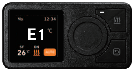
Temperature sensor short circuit
